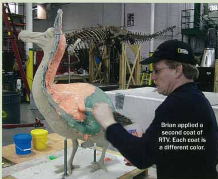
38. Two more coats of RTV rubber were applied to give the inner mold strength. Pulling the casts from the mold can cause it to tear if the rubber is not thick enough. Since the second and third coats do not come into contact with the sculpture, they do not need to be vacuumed, but a fixitrope was added to the RTV rubber to make it thick and brushable. Each coat was a different color, which helps the mold maker ensure complete coverage of each successive coat.
