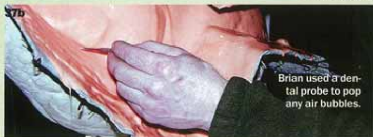
37b. Brian used a dental probe to pop any bubbles that formed on the surface of the RTV rubber before it cured.
