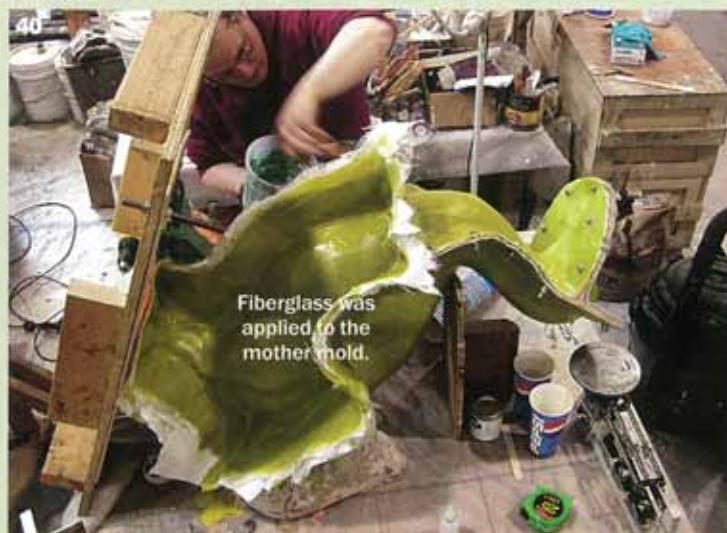
40. Once the RTV rubber cured on the first section of the mold, Brian covered it with a layers of fiberglass cloth soaked in epoxy. This epoxy shell, which gives the mold its structural integrity, is called the "mother mold."
